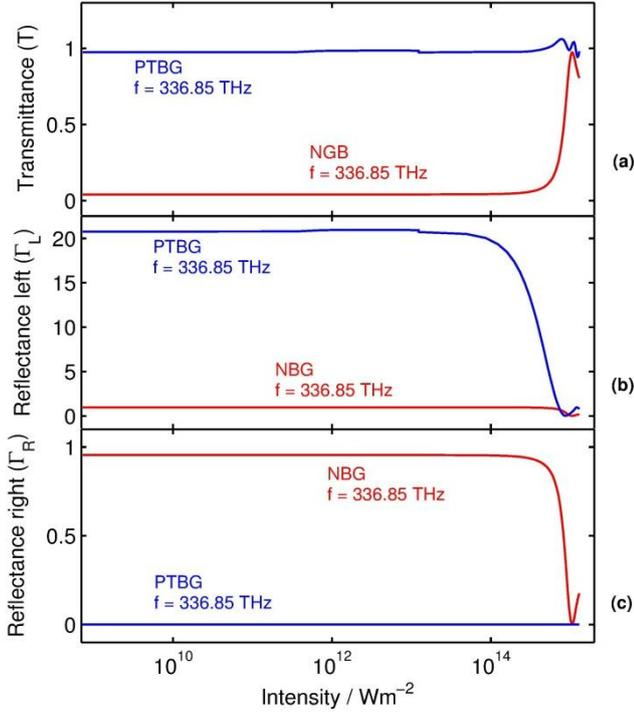
Fig. 4 (a) Transmittance, (b) reflectance for left and (c) reflectance for right of PTBG at the U operation as a function of input intensity at  $f = 336.85 \text{ THz}$ . The gain/loss has high saturation intensity  $n_2 I_S = 0.5$ . Results for the NBG ( $\alpha_0 = 0$ ) at the Bragg frequency  $f_B = 336.85 \text{ THz}$  are included for reference.
