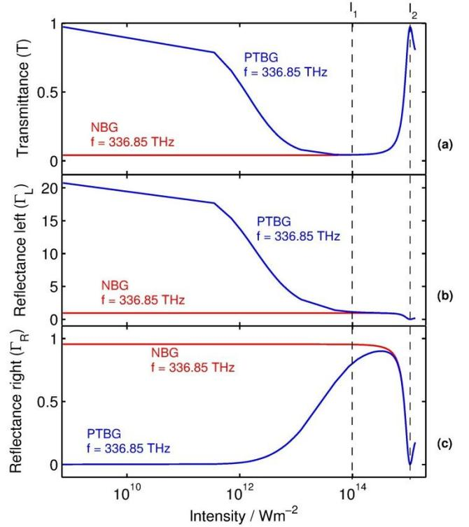
Fig. 5 (a) Transmittance, (b) reflectance for left and (c) reflectance for right incidence of PTBG at the U operation as a function of input intensity at  $f = 336.85 \text{ THz}$ . The gain/loss has low saturation intensity  $n_2 I_S = 0.0005$ . Results for the NBG ( $\alpha_0 = 0$ ) at the Bragg frequency  $f_B = 336.85 \text{ THz}$  are included for reference.
