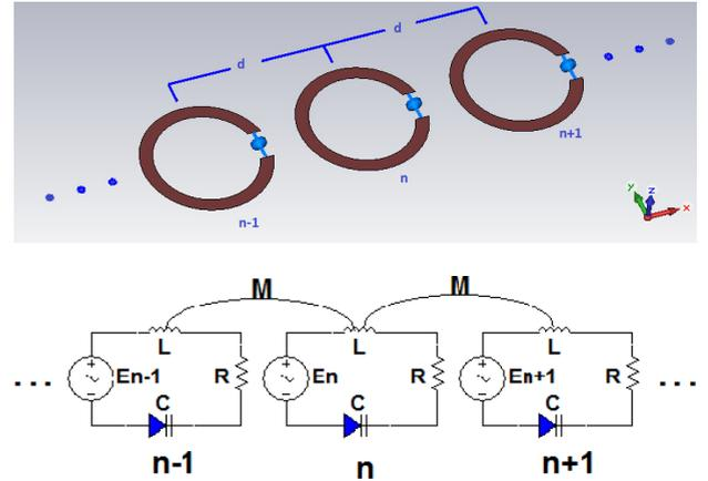
Fig. 1. (Top) A representative illustration of the nonlinear magnetic metamaterial structure. (Bottom) The equivalent circuit model (see text for details).
