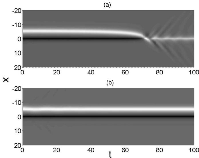
Figure 4. Evolution of the solution  $SF^{(3)}$  shown in Fig. 2 with  $\alpha = 0.01$  is presented in terms of the magnetic field  $\phi_x$ . (a) The solution is unstable. We see the collision of a  $2\pi$ -fluxon (bright line before  $t \approx 75$ ) and an anti-semifluxon (dark line) producing a semifluxon (bright line after  $t \approx 80$ ). (b) The stabilization of the solution by a defect.
