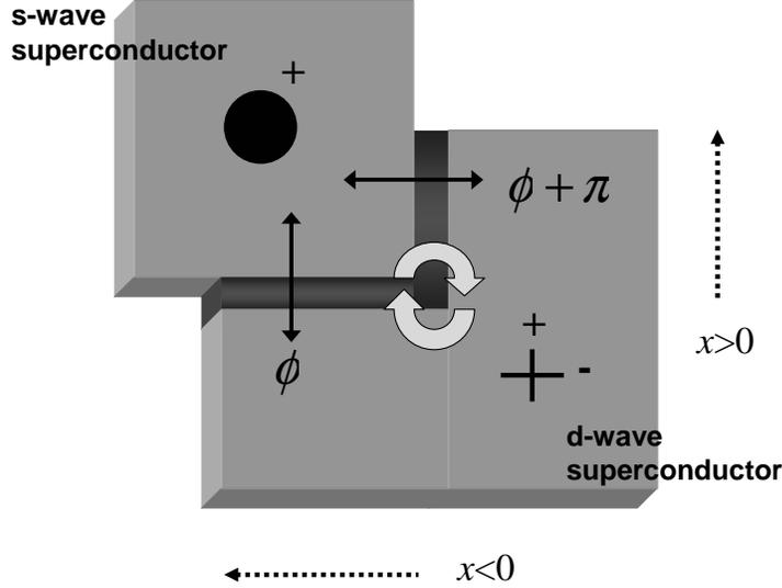
Figure 1. A sketch of a corner junction made by two superconductors, i.e., an s-wave superconductor (low- $T_c$  superconductor) and a d-wave superconductor (high- $T_c$  superconductor). A circulating current with a half-flux quantum, or semifluxon, is created and attached to the discontinuity point.
