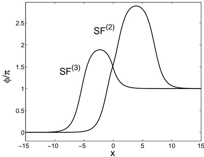
Figure 2. The plot of the two non-monotone semifluxons for  $\gamma = 0.01$ . The solution with the higher and lower hump is denoted by  $SF^{(2)}$  and  $SF^{(3)}$ , respectively.
